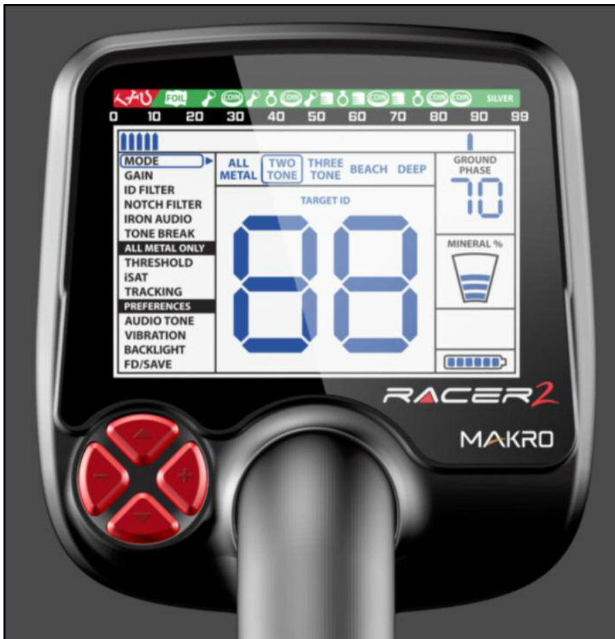
The Racer 2's screen not only provides a lot of valuable target ID information, but also allows fast mode changes and adjustments.
