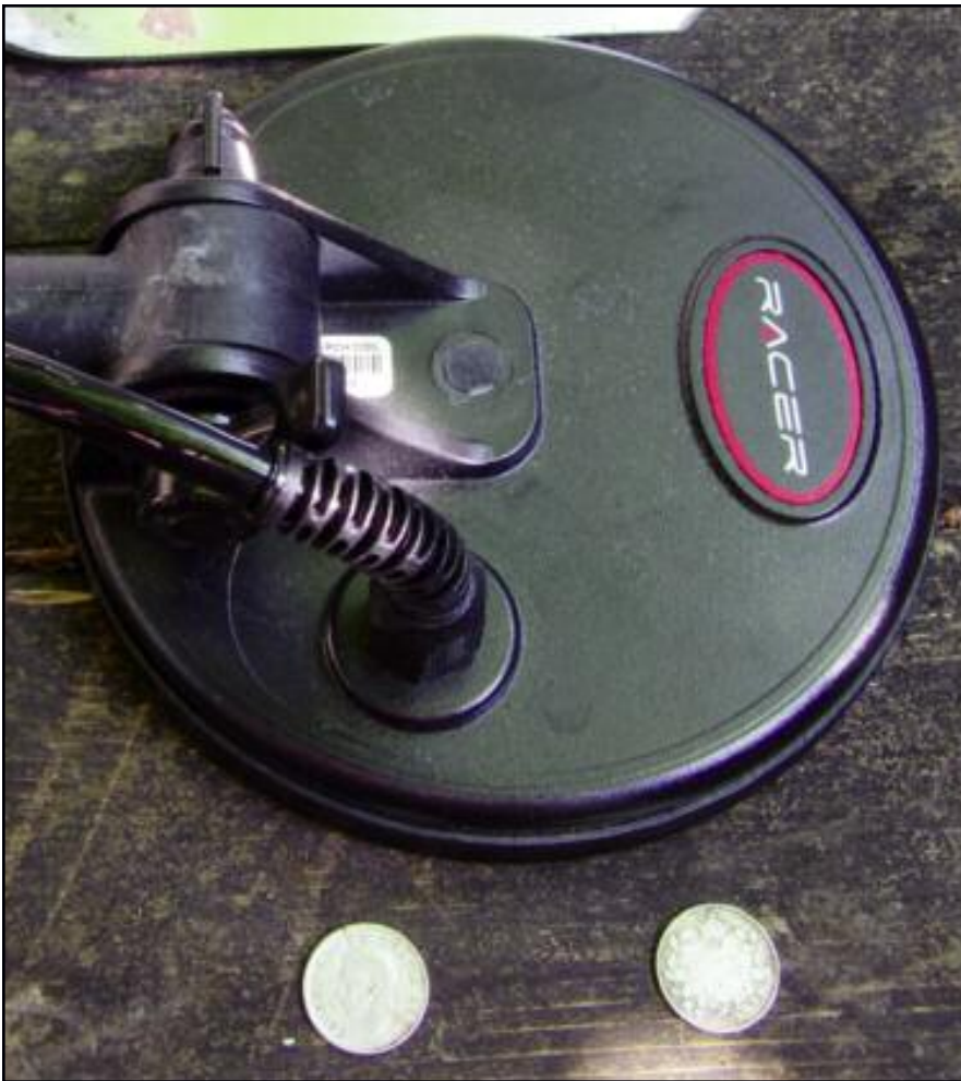
The RC13 DD 5" coil combines well with the Racer 2's tone ID features to bring up silver signals in iron-infested sites.
