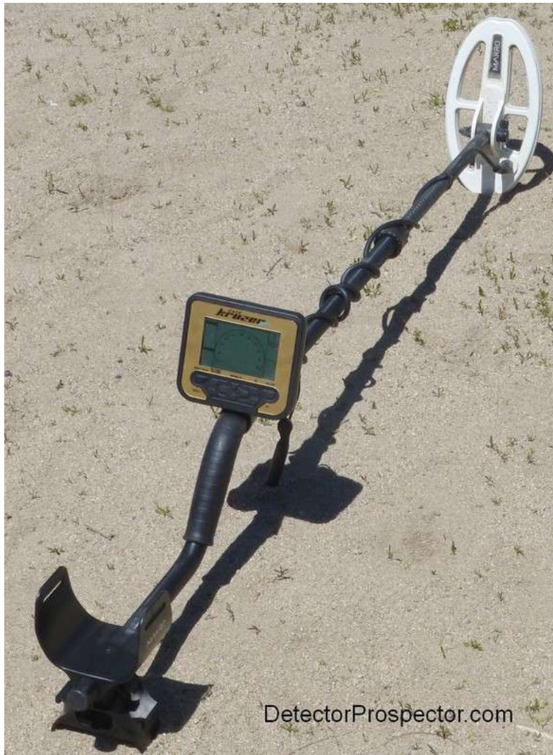
Makro Gold Kruzer with optional 5" x 9.5" DD coil
