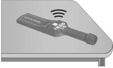
When the device is laid down flat on a surface that contains metal with the indicators facing up, it will go into an auto stand-by mode right after emitting an alarm for a second.
