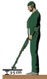
6. If there is no ground effect on the device there is no interaction on the bar that is indicated in the figure and “Ground Setting 100% Completed” expression is displayed. In this case the device is ready for exploring and you may switch to explore mode by pressing the “ACCEPT” button.
