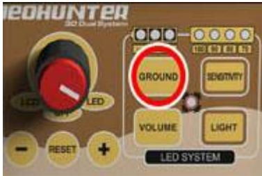
1. To make ground setting the device is turned on in “LED” mode and “GROUND” button is pressed.
