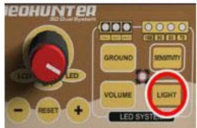
After pressing the Light key the level of illumination is adjusted by pressing “+” and “-“ keys. After the illumination level is set “Light” key is pressed again to switch to Explore mode.
