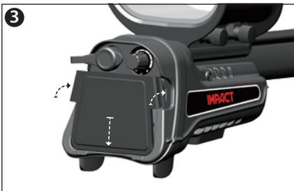
Place the battery cover in the direction of the arrow shown in the picture. Push down on the tabs to get the cover click into its place.
