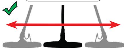
It is important to keep the search coil parallel to the ground in order to get accurate results.
