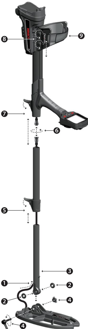
(1) Insert the search coil cable through the hole at the back of the lower shaft.
