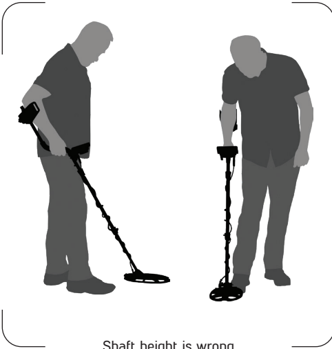
Shaft height is wrong
