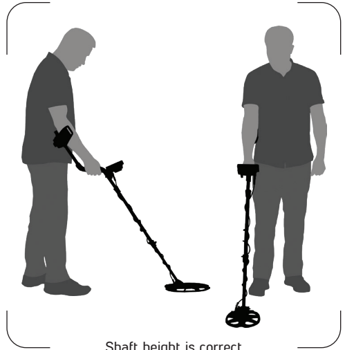
Shaft height is correct
