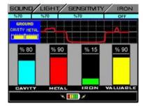
Ground effect that may be formed together with the target is also displayed on the display.
