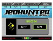
again. After this operation press "SETUP" button to switch to the previous mode. Following this step the device will filter worthless metals. To be able to detect worthless metals again this mode should be switched back to "ON" mode by repeating above mentioned operation.
