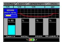
If the target is a CAVITY, there is a raise on the "CAVITY" bar and decrease in the graph. The intensity of the "CAVITY" bar is indicated as % on top depending on the magnitude of the effect of target.  If the target is valuable metal, there is a raise both on the "METAL" and "VALUABLE" that is expressed in % depending on the magnitude of the effect. The effect of metal can be monitored in the graph on top of the bars.
