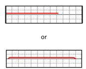
If the signal line increases very sharp and decreases with same velocity there is no need to calculate depth. Because, this shows that the target is very close the surface. Oscilloscope never draws a straight line while it receives signals from true target, it always draws sinuous lines. Oscilloscope line is closer the center line when the target is deep and line is away from the center line when the target is close.
