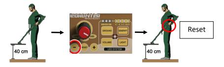
If the ground settings cannot be realized by above described operations, "SENSITIVITY" level of the device should be decreased one step and above mentioned operations are repeated.
