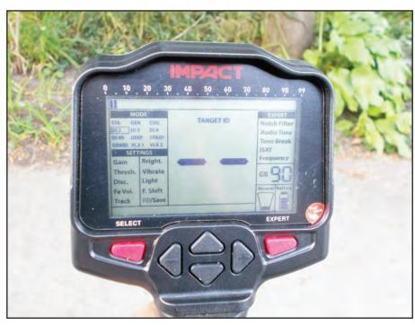
The Impact's screen provides easy access to all of its features without complicated menus. Real-time information on ground condition, battery strength, and target composition are also shown on the screen. Backlighting allows it to be used in low and no-light conditions.
