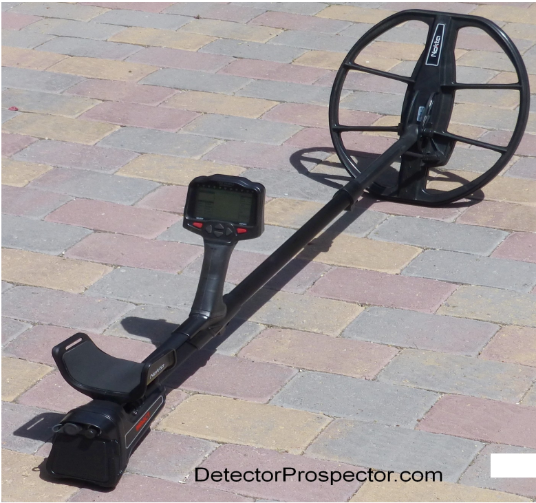
Nokta Impact with IM40 15.5" x 13.75" coil mounted
